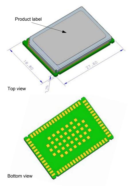
Figure 2: BGS2-E/BGS2-W- top and bottom view
